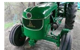
Schlepper **D5505** 4Zyl. 52Ps 8+4Gang-Getriebe, Ber. 11-36AS
